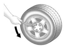
To remove the plastic covers and wheel nut caps, loosen the plastic nut caps with the wheel wrench in a counterclockwise direction. If needed, finish loosening them with your fingers. The plastic nut caps will not come off.
